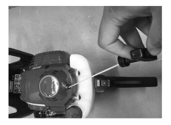
If engine starting is not obtained, put the choke lever on the position and pull again the recoil handle
